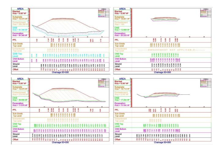
These are some examples of Cross-Sections which are drawn by my Excel based program to plot on Auto CAD and we can modify the properties of Cross-Sections as per our requirement.
